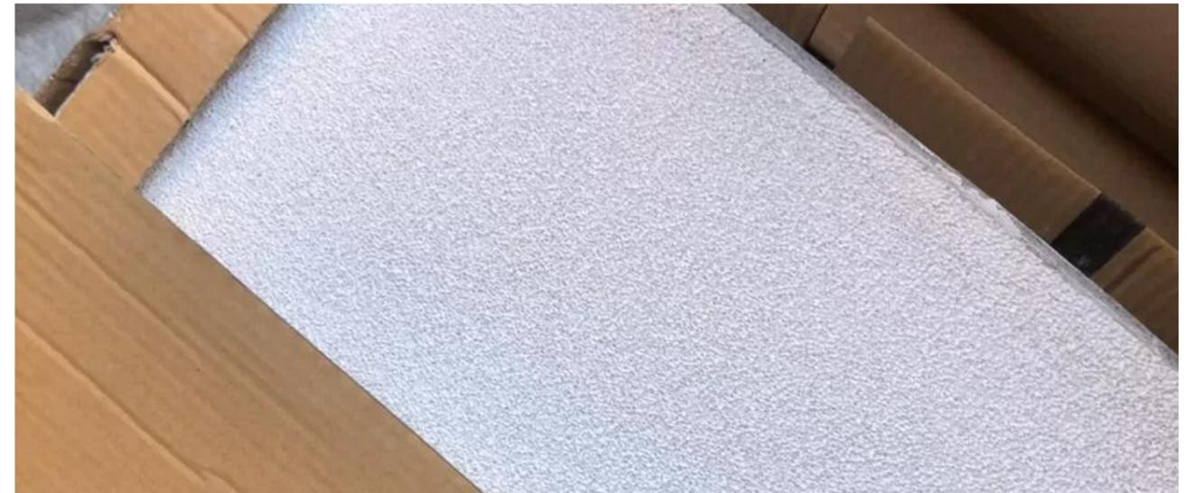
Our Silicon Carbide Ceramic Foam Filter employs German-imported polyurethane foam sponge as a carrier, infused with silicon carbide. This innovative process involves embedding the foam sponge with a slurry of silicon carbide, which forms a robust ceramic structure after drying and high-temperature baking. The decomposition of polyurethane leaves behind a highly efficient filtering medium.
